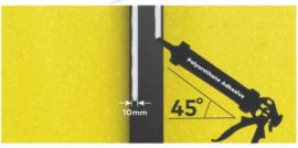
3. Applying polyurethane adhesive on the vertical profile
