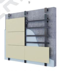
Invisible mechanical fixing system with anchors stages
