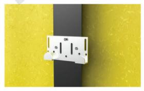
2. Installation of bottom fixing clips on vertical profiles
