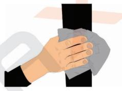
1. Cleaning and drying of vertical profiles
